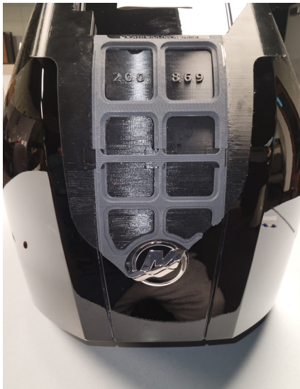
3D printed FDM decal application fixture shown on a marine engine cover.
